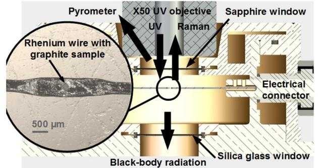
Figure 2: Sectional view of the wire-loop heating stage. The zoom is a picture of the heating rhenium wire with the sample confined in a 400  $\mu\text{m}$  of diameter hole. Pyrometric and UV Raman measurements are performed alternatively through the sapphire window. Black-body radiation can be recorded simultaneously in the 400-1200 nm range through the silica glass window at the bottom of the cell.
