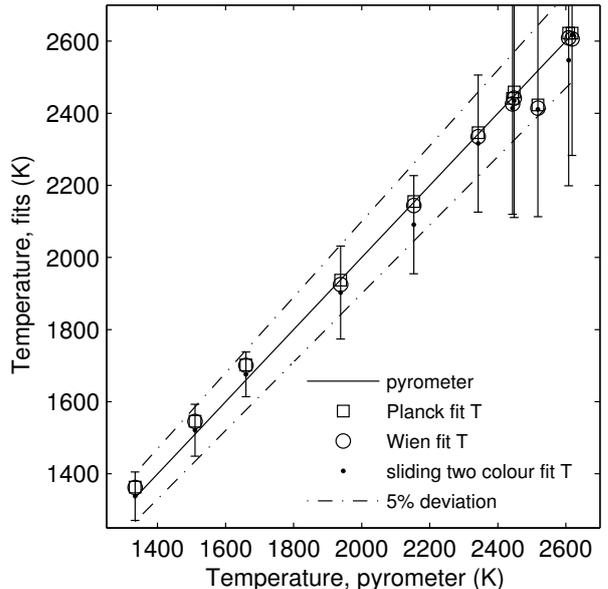
Figure 3: Comparison of temperature fits of thermal emission spectra with pyrometric measurements. The solid line is the 1:1 correlation. The errors for Planck and Wien fits are within the symbol size ( $\square$  and  $\circ$ ). The dot dashed lines indicate  $\pm 5\%$  deviation from pyrometry temperature.
